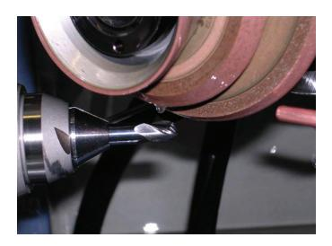
"Fives, pioneering Gardner Abrasives solutions for the re-sharpen of cutting tools in various complex geometries."
